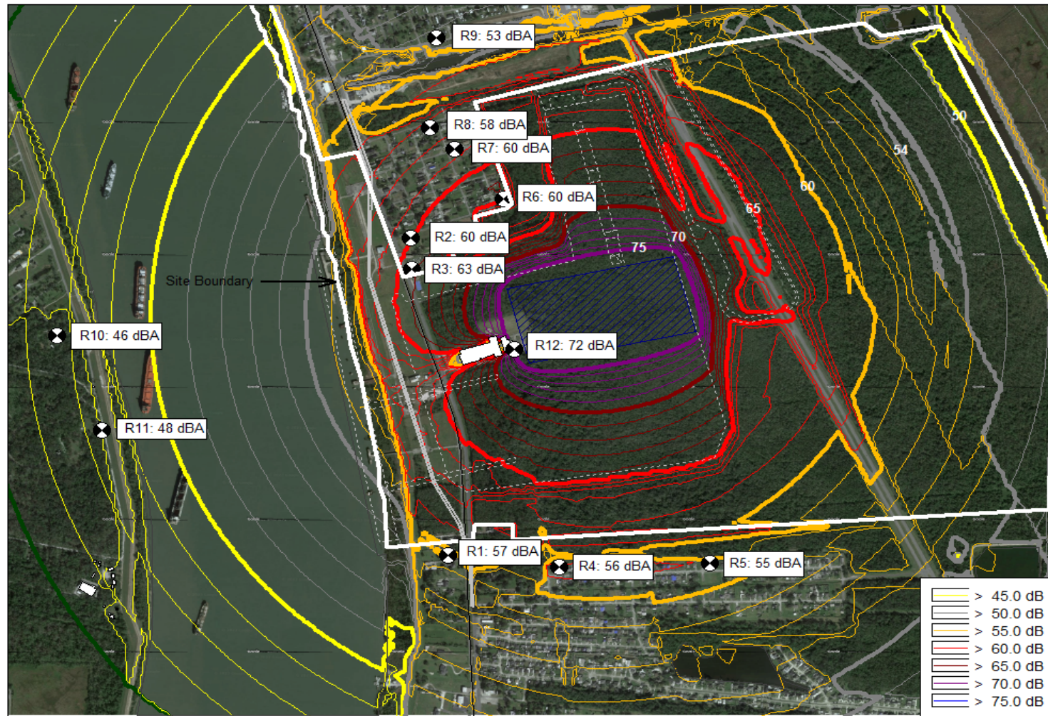
Figure 3. Airborne Sound Contours During Phase 2 Daytime Construction
